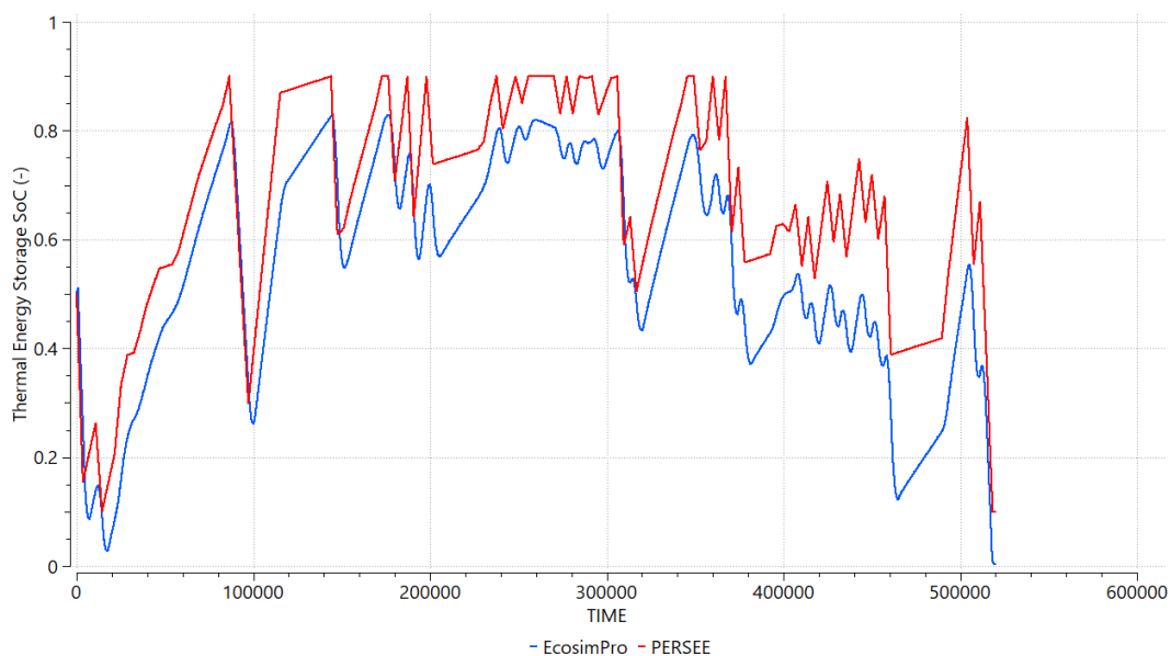
Figure 18: TES state of charge – EcosimPro® vs PERSEE
